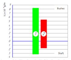
**Fig. 11:** Diagram of the Wear Intensity U of the Coupling Parts during the Different Methods of Bushes Treatment (Wear Limit). 1- Reaming Treatment; 2- Vibro-Rolling Treatment Followed by Broaching Deformation.
