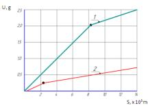
**Fig. 10:** Dependence of Wear U of the Bushes According to the Friction Distance S: 1 - Reaming Treatment; 2 - Vibro-Rolling Treatment Followed by Broaching Deformation.
