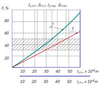
Fig. 7: Dependence of the Bearing Surface F of the Treated Area by Vibro-Rolling According to the Magnitude of the Convergence Value  $\Delta$  (1) and the Treated Surface by Vibro-Rolling after the Broaching Deformation Depending on the Allowance J<sub>Im</sub> (2).
