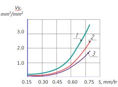
**Fig. 6:** Dependence of Surface Specific Oil Absorption Vy MR According to the Advanced Movement S during Different Diameters of the Ball Db(1 - Db= 3.97 mm; 2 - Db= 5.80 mm; 3 - Db= 7.94 mm).
