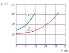
**Fig. 14:** Temperature T Dependence of the Friction Area According to Oil Retention Forces P during Different Treatment Methods. 1 - Reaming Treatment; 2- Vibro- Rolling Treatment Followed by Broaching Deformation.
