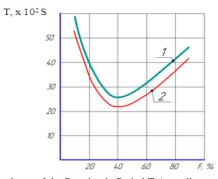
**Fig. 9:** Dependence of the Running-in Period T According to the Bearing Area F after by Broaching Deformation. Shaft: Tempered Steel 45; Untempered Steel 45; Bushes: 1, 2 - Br OCS 5-5-5.
