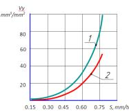
Fig. 5: Dependence of Surface Specific Oil Absorption Vy MR According to Advanced Movement S at Different Amplitudes of the Oscillations L of the Roller (1 - L = 5 mm; 2 - L = 10 mm).
