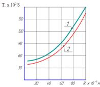
**Fig. 8:** Dependence of the Running-in Period T According to the Height R of the MR Element after the Vibro-Rolling: Shaft: Tempered Steel 45; Untempered Steel 45. Bushes: 1, 2 - Br OCS 5-5-5.
