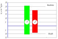
**Fig.12:** Diagram of the Wear Intensity U of the Coupling Parts at Various Methods for Surface Treatment of the Bushes (Dry Wear). 1 – Reaming Treatment; 2 - Vibro- Rolling Treatment Followed by Broaching Deformation.
