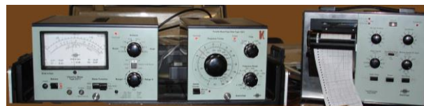
Fig. 3. A set for wear rate study by measuring the acoustic signal amplitude.
