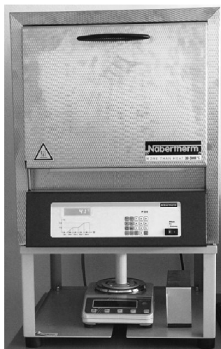
Figure 2 – Gravimetric furnace Nabertherm L9/11/SW/P330
