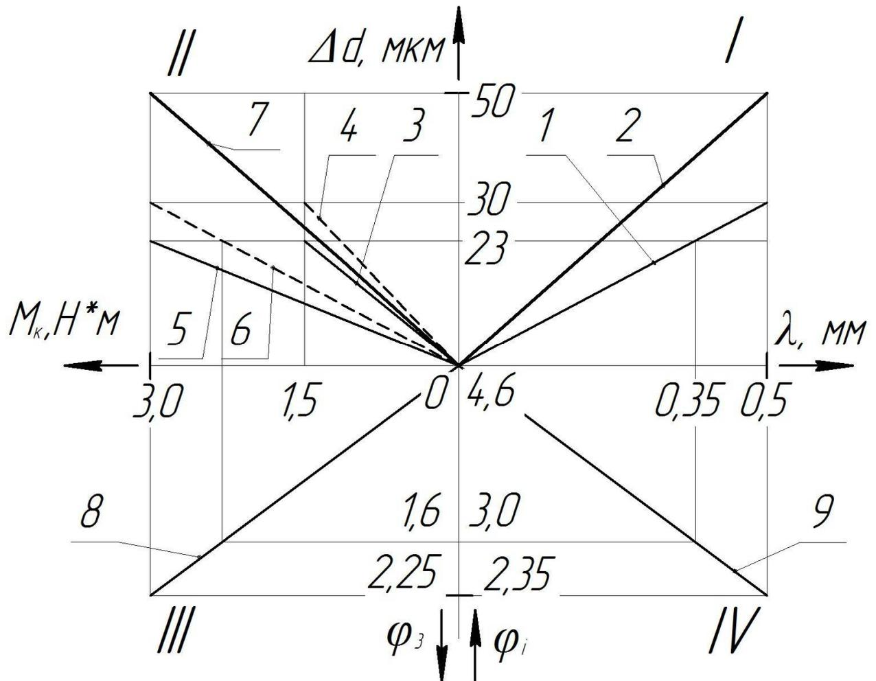
I – theoretical 1 and experimental 2 dependence  $\Delta d=f(\lambda)$ ; II – theoretical 3,4,5,6 and experimental 7 dependences  $\Delta d=f(M_k)$ ; III – theoretical dependence 8  $\varphi_3=f(M_k)$ ; IV – theoretical dependence 9  $\varphi_3=f(\lambda)$ ;  $\Delta d$  – diameter increase;  $M_k$  – torque;  $\lambda$  – axial draft of HSDS;  $\varphi_3$  – twisting angle;  $\varphi_i$  – alternating value of the angle of the screw line lifting;
