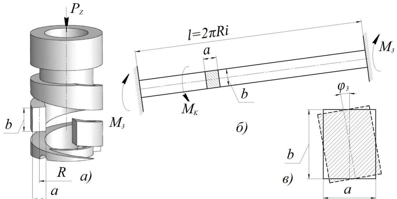
$R$  – HSDS radius;  $P_z$  – compressing force;  $M_3$  – closing moment;  $M_k$  – torque;  $\varphi_3$  – angle of twisting the cut;  $i$  – number of complete spirals of HSDS;  $l$  – length of spirals;
