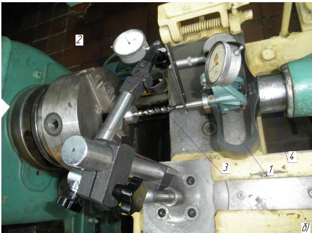
1 – dynamometer; 2 – magnetic indicator stand; 3 – HSDS; 4 – tailstock pinole;
