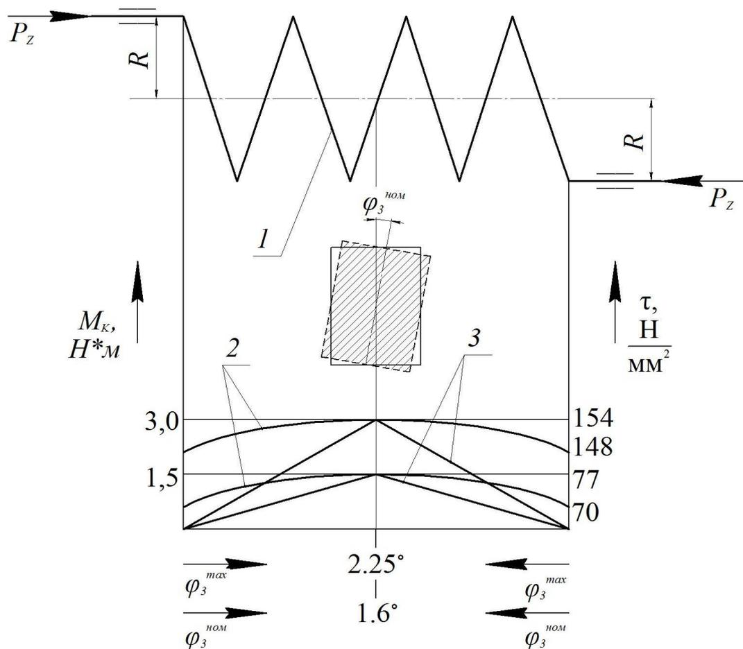
1 – HSDS; 2 – curvilinear dependence of the change of tangent tensions  $\tau$  along the body of HSDS received by the method of computer diagnostics; 3 – the area of adjacent triangles which reflect the operation of the torque  $M_K$ .
