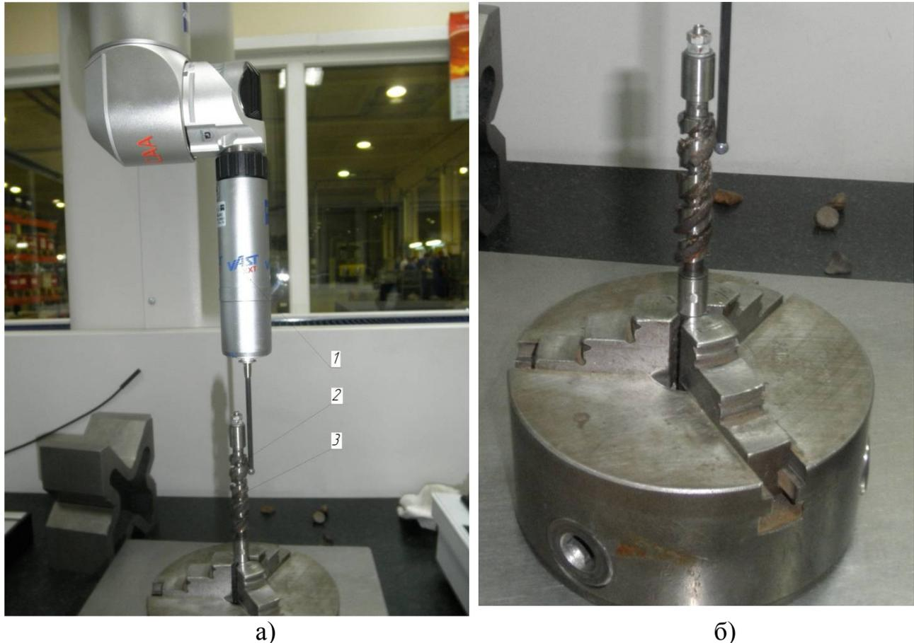
1 – the reference machine Carl Zeiss CONTURA G2; 2 – sensor; 3 – HSH.
