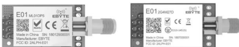
Figure 2 - Transceivers E01-ML01DP5 and E01-2G4M27D
