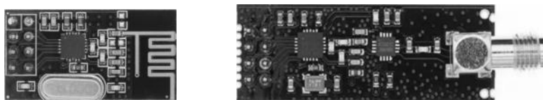
Figure 1 - NRF24L01+ and NRF24L01+PA+LNA transceivers
