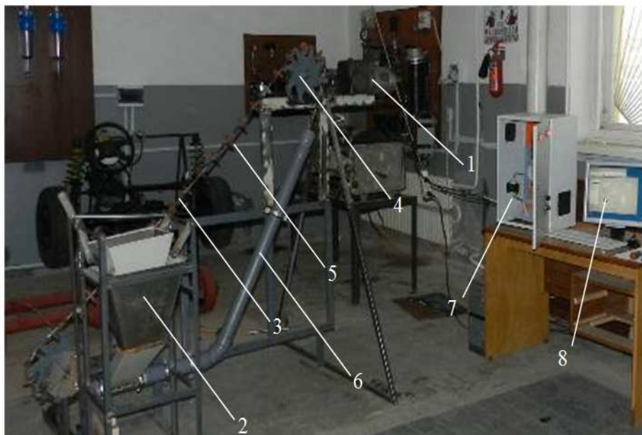
Fig. 5. General view of the experimental setup: 1 - conveyor drive; 2 - filling hopper; 3 - working body of the tubular scraper chain conveyor; 4 - drive sprocket; 5 - scraper; 6 - transport way; 7 - frequency converter; 8 - personal computer.
