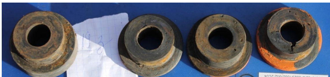
Fig. 9 - General view of experimental details of the upper lever after testing in parallelogram mechanism of cultivator
