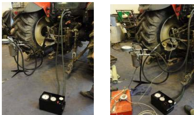
Figure 5 – Filter device, Owatonna device and CS 1000 optical device connecting to a hydraulic outside circuit of tractor
